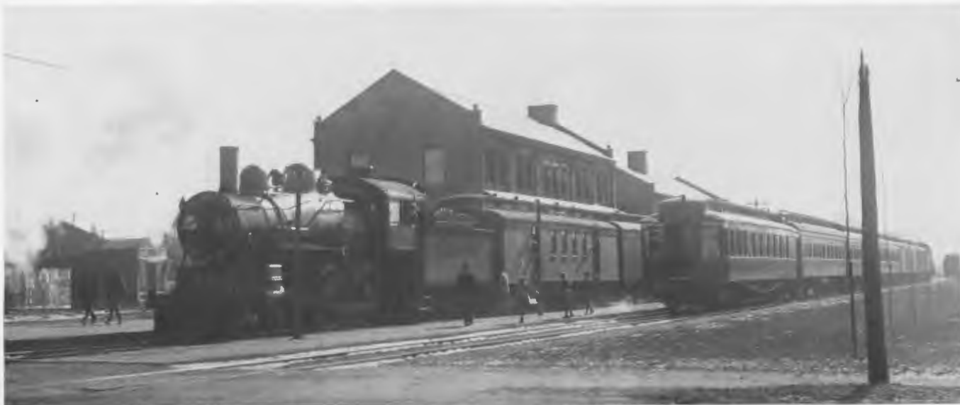
In a tradition that continued for another forty years, trains 116 and 117 are shown here laying over for lunch in 1907. Apparently, train 117, pulled by engine 211, a class B, 4-4-0 type, has just arrived and there are some moves to be made. Her fireman appears to be anticipating a signal from a man who is stepping between the tender and the Railway Post Office car. The three young lads on the platform seem to know just where the action is. Photo from the collection of Russ Porter.
