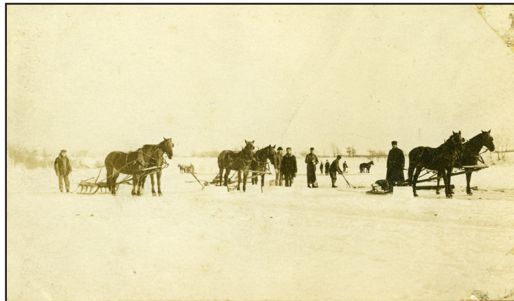
Healy's crew cut blocks of ice out of Kellogg's Pond and teams of horses hauled them to his storage warehouse just off Fifth Ave. near the lake.
